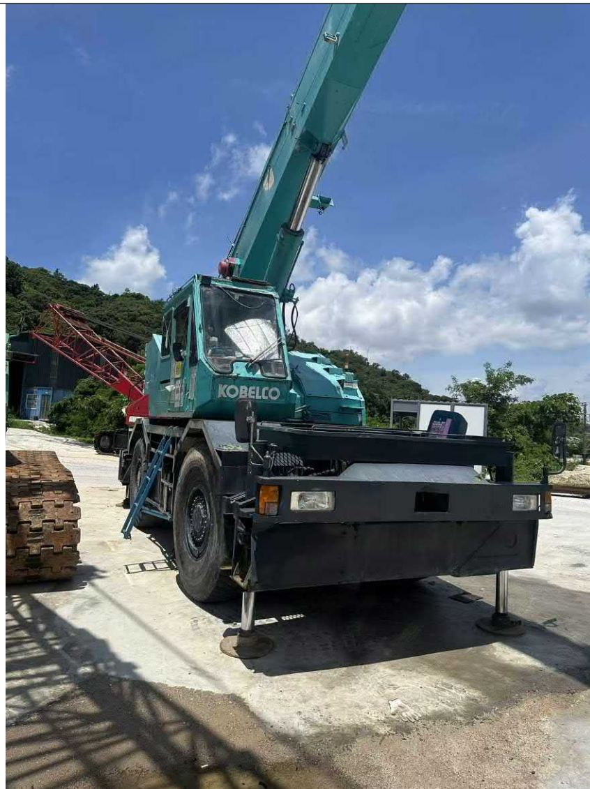
Figure 1: Wheeled hydraulic telescopic boom crane for supervised training and examination preparation; any future official testing at the Site is subject to separate Labour Department approval.
